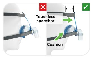
When adjusting the fit of your mask, ensure the touchless spacebar DOES NOT contact the forehead when tightening the top straps.
